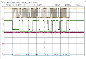
No acknowledge (NACK) from the master after reading out the  $5^{\text{th}}$  data byte. The "Missing Ack" that is recorded in the tables is not a mistake, it's a must.
