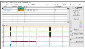
The EOC line is low for 7.75ms. The newest datasheet guarantees a conversion time below 8ms, typ. 6ms. To reach sample rates over 100 SPS it is a must to work with a high bit rate and to check the EOC line or to poll the STATUS byte.
