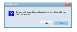
The reason to offer this communication tool is to make the changing of the slave address as easy as possible. The memory technology of the D-Line transmitters is one time programmable (OTP). There are 4 pages of one time programmable memory. That means, that it is a must to do the copy job 'right first time', the "D-Line Address Manager" can do all of that for you.
