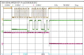
Nice to see: The ACK from the slave follows immediately to the negative edge of the 8th clock impulse (two times visible).
