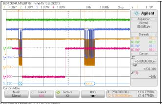
The simplest way to "detect" the end of a conversion (EOC) is to wait until the new data is definitely ready to read out. Being on the safe side; the conversion and the conditioning of the pressure and temperature value is completed after 8ms.
