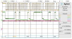
More detailed view of the readout frame: EOC is back to 3.6V. The slave ACK occurs as normal immediately after the neg. edge of the 8<sup>th</sup> clock impulse. The ACK from the master occurs with a little delay but this is allowed because the master generates the 9<sup>th</sup> clock impulse by itself at the right time.
