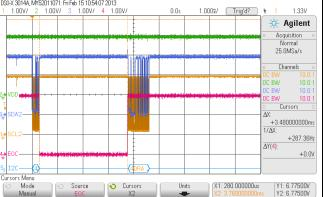
The handshake-solution, done by the additional EOC wire, is very elegant and is suitable to save time and power. The Master controller can be in sleep mode and will be awoken by an external interrupt on the positive slope of the EOC pin. Polling the level of the EOC wire is also possible.
